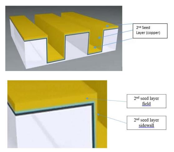
A second seed layer is deposited by a PVD technique over the first seed layer. The second seed layer is thicker than the first seed layer over the field.
