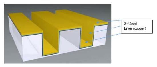
A PVD chamber is used to deposit a second seed layer over the substrate.
