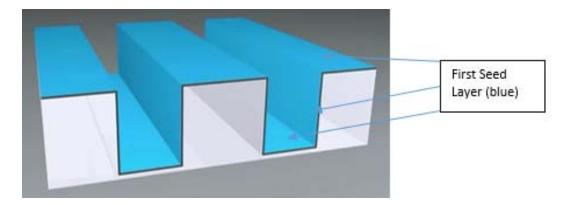
A CVD chamber is used to deposit a first seed layer over the sidewalls of at least one
