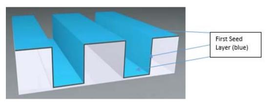
a. depositing a substantially conformal seed layer over the field and inside surfaces of the at least one opening;
