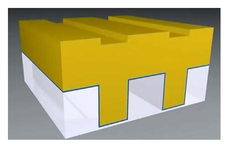
61. After the electroplated copper is disposed over the openings and the field, the electroplated copper overlying the field, the first and second seed layers overlying the field, and the barrier layer overlying the field are all substantially removed by a polishing technique. The resulting interconnect is as is depicted below.
