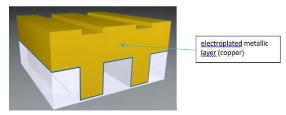
After the substantially non-conformal seed layer is applied through a PVD process, an electroplated metallic layer of copper (i.e. "Cu") is disposed over the substantially non-conformal seed layer.
