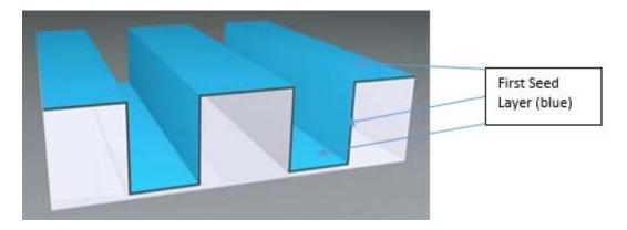
A first seed layer is deposited by a CVD technique over the barrier layer.
