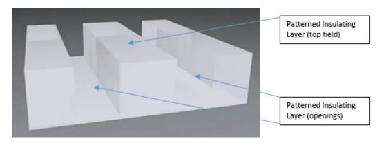
c. a barrier layer disposed over said patterned insulating layer including over inside surfaces of the at least one opening, as depicted below:
