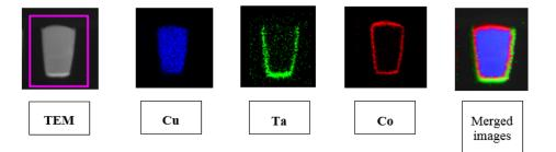
64. The presence of a cobalt ("Co") seed layer in these cross-sections confirms the use in the Accused Chips of the multiple-seed-layer process described above.
