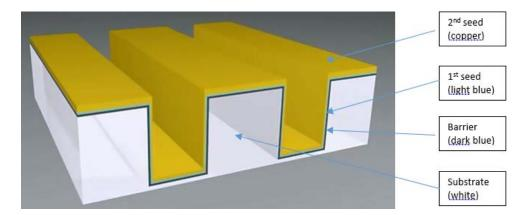
60. After the barrier, first seed layer and second seed layer are formed over the substrate, electroplated copper is disposed over the second seed layer over the openings and the field, as depicted below.
