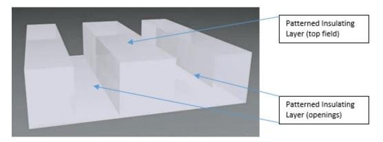
b. depositing a barrier layer over the field and inside surfaces of the at least one opening, as depicted below;
