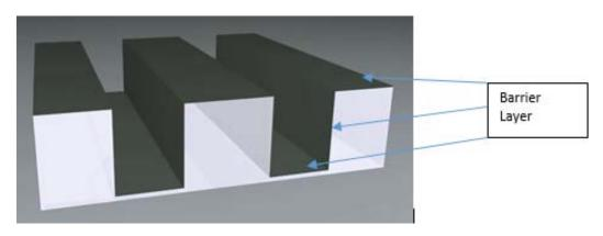
In the case of the Accused Chips, tantalum nitrite is used for the barrier layer and is applied through a PVD process.
