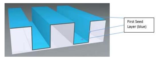
A first conformal layer of cobalt is applied over the barrier layer through a CVD process.
