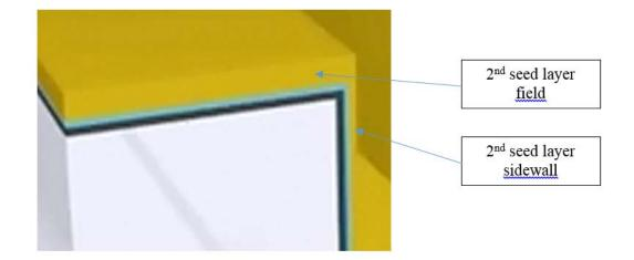
As is now well known in the art, at the geometries found in the accused chips, an optimized PVD copper seed layer at the 2x nanometer node and beyond will result in sidewall coverage at midpoint of about 13% to 15% of the thickness on the field, and certainly less than 25% of the thickness on the field.
