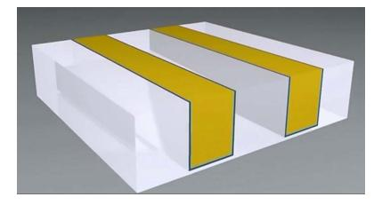
As explained in the Volta Animation, after copper is used to fill the openings and applied over the field through electroplating, the copper over the field and the barrier layer and first and second seed layers over the field are removed using a polishing technique.
