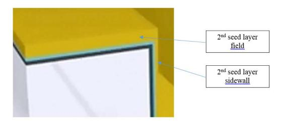
As depicted above and on information and belief, an optimized PVD copper seed layer at the 2x nanometer node and beyond will result in thickness over the field far greater than that of a substantially conformal CVD seed layer. Further, as depicted in the Volta Animation, the substantially conformal and the substantially non-conformal seed layers do not seal the at least one opening.
