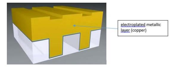
The openings are filled by electroplating copper over the two seed layers.
