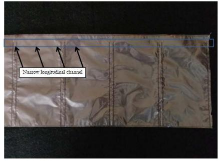
The Accused Automated EZ-Tear Webs have at least one row of generally rectangular presealed inflatable chambers each having three sides closed and a fourth side with an unsealed opening into the longitudinally extending channel (for example, as shown below, the DuraClear 2000 EZ-Tear Pillows define three closed sides and fourth unsealed side for inflation).
