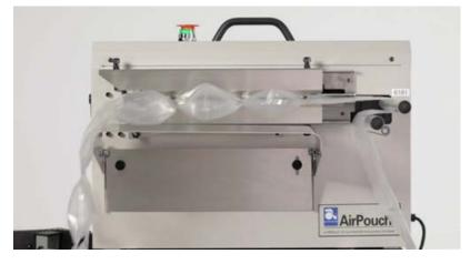
42. The Accused Automated System contains a feed mechanism that causes the plastic film to be gripped at or near the narrow longitudinally extending channel and drawn in a continuous and uninterrupted manner through inflation, sealing and slitting mechanisms in a planar path (for example, the AirPouch® Express 3™, as shown below, contains a feed mechanism that pulls in the film having a sealing and slitting mechanism in a planar path).
