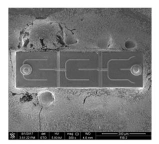
99. Below is a scanning electron microscope image of a pair of holes milled into the LED chip using a focused ion beam.
