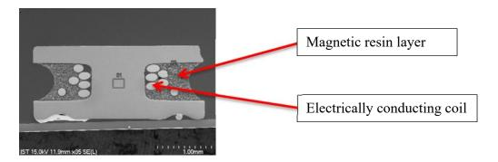
14. The magnetic resin layer contained in the Accused Inductors contains a magnetic powder dispersed in a polymer resin. The spectrum below indicates that the magnetic resin layer contains approximately 35% iron (Fe), a magnetic substance, and approximately 51% carbon (C), that is used for the polymer resin.
