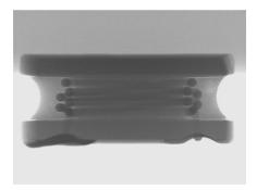
13. The Accused Inductors comprise a magnetic resin layer compression-molded to embed at least a portion of an outer periphery of said electrically conducting coil. On information and belief, the resin layer is compression-molded.
