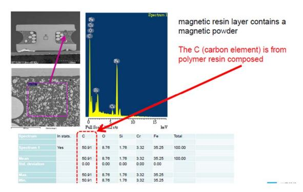
The following spectrums detail the individual components of the magnetic resin layer. Spectrums 1 and 2 indicate the presence of a ferromagnetic metal powder, iron (Fe). Spectrum 3 indicates the presence of the polymer resin.
