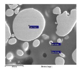
Spectrum 1 & 2: ferromagnetic metal powder Spectrum 3: polymer resin
