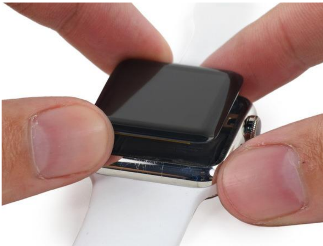
Figure 32: Photo of Apple Watch screen removal, Ex. 73.
