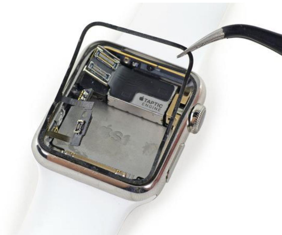
Figure 33: Photo showing Apple Watch force sensor ring placement, Ex. 74.
