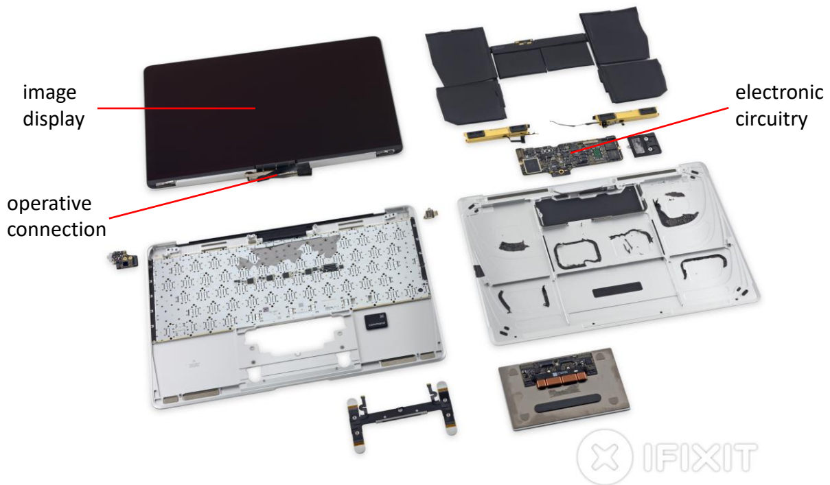
Figure 13: Teardown view of a MacBook, with labeling added, see Ex. 30.
