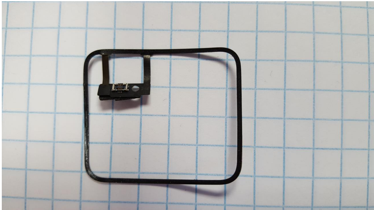
Figure 34: Photo showing Apple Watch force sensor ring, Ex. 75.
