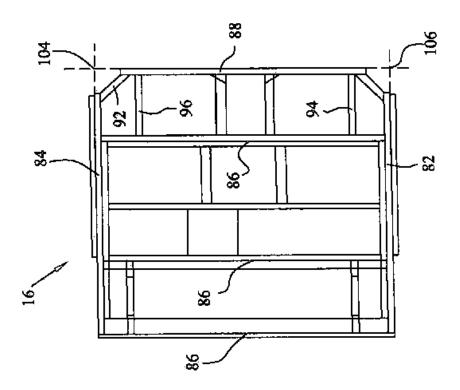
By comparison with the prior types of chassis, the front corners (denoted by numbers 104 and 106), have been formed with angled beams (denoted by numbers 90 and 92) connecting the front beam of the chassis (denoted by number 88) with the respective side beams of the chassis (denoted by numbers 82 and 84). A perspective view of the front of the chassis taken from Figure 10 of the '251 patent illustrates this arrangement as:
