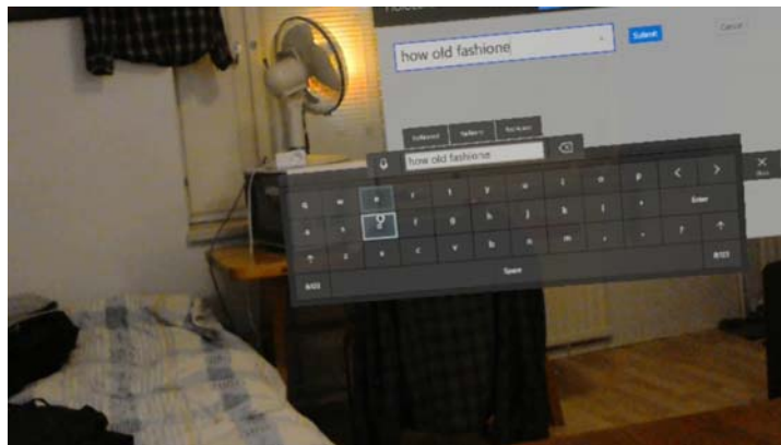
Figure 2 - Operation of Holographic Keyboard on HoloLens
