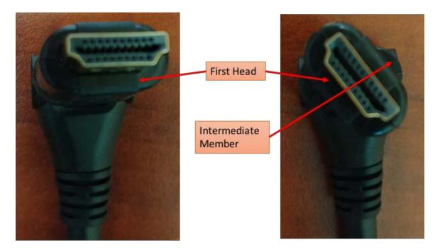
28. Defendant's Accused Products comprise a first electronic connector on the first head connectable to a first electronic device. For example, the representative VisionTek 1 Meter High Speed HDMI to HDMI Pivot Cable has an electronic HDMI connector on the first head as shown below.
