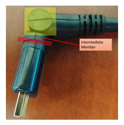
21. Defendant's Accused Products comprise a first head rotatably connected to the first end of the intermediate member and limited to rotation in a first plane on the first connection axis. For example, the representative VisionTek 1 Meter High Speed HDMI to HDMI Pivot Cable has a rotatable head attached to the intermediate member that rotates as shown below.
