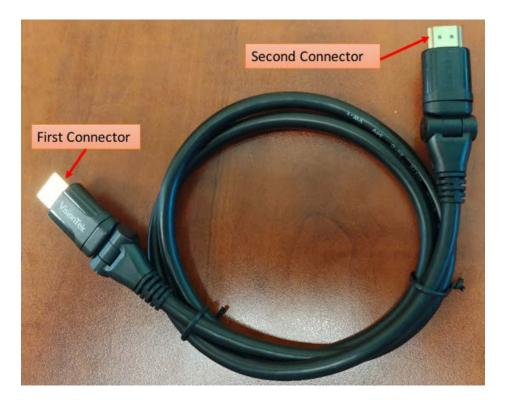
25. Defendant's Accused Products have at least one of the first and second heads to be rotatable on its connection axis more than 90-degrees relative to the intermediate member. For example, the representative VisionTek 1 Meter High Speed HDMI to HDMI Pivot Cable can rotate about the second connection axis 180-degrees relative to the intermediate member as shown below.
