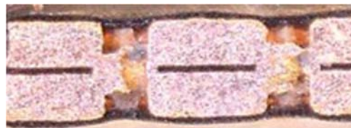
Samsung Note 5 Wireless Power Coil Released August 2015 (Cross-section showing double conductive layer)
