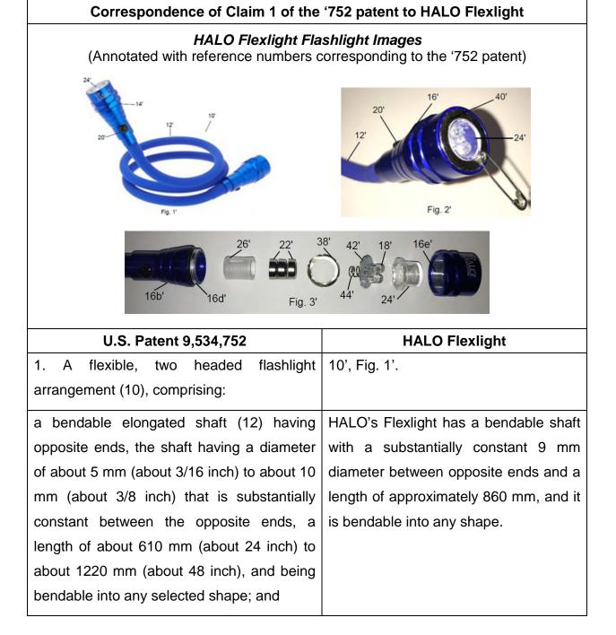
a separate self-powered flashlight assembly (14) fixed to each end of the shaft (12), each flashlight assembly comprising a housing (16) containing an LED circuit with at least one LED (18), a switch (20) having open and closed positions for respectively interrupting and passing electricity to the LED (18) and at least one battery (22) for powering the LED when the switch is closed;
