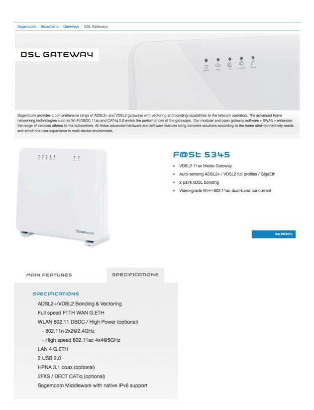
Figure 1. The F@St 5345 is compliant with IEEE 802.11ac and 802.11n wireless distribution systems, and therefore provides a customer premises system.
