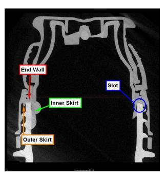
20. The slot of the Accused Instrumentality receives the container rim when the closure is applied to the container and is in a sealing position:
