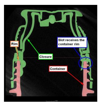
21. The inner skirt of the closure of the Accused Instrumentality has a deflecting section in the region of the free end of the inner skirt, and a sealing section spaced from the deflecting section:
