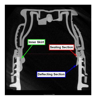
22. Between the deflecting and sealing sections of the closure of the Accused Instrumentality, there is a space between the inner skirt of the closure and the inner surface of the outlet of the container:
