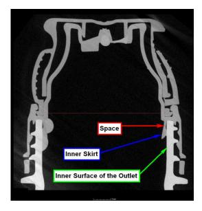
23. The cross-sectional area of the deflecting section of the closure of the Accused Instrumentality is greater than the cross-sectional area of the inner surface of the outlet of the container such that when the closure is applied to the container, the deflecting section of the inner skirt engages the inner surface of the outlet and causes a deflection thereof:
