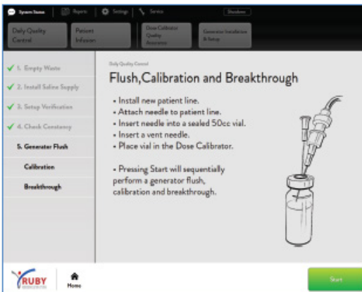
Figure 49, Flush, Calibration, and Breakthrough Screen
