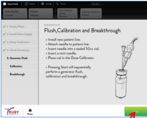
Figure 49, Flush, Calibration, and Breakthrough Screen
