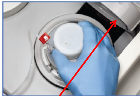
Figure 7, Waste Bottle in Waste Well
