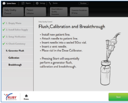
Figure 49, Flush, Calibration, and Breakthrough Screen
