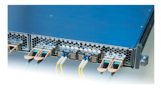
Fiber input and output ports used to connect fibers to transceivers are also present in the exemplary Flashwave 9500 product, as shown in the figure below.<sup>33</sup>
