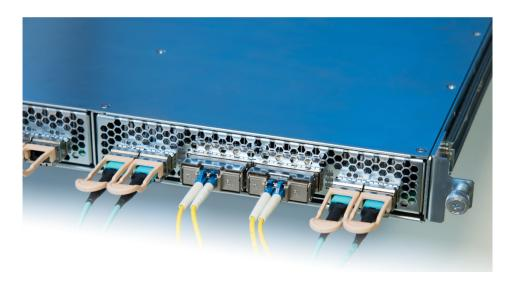
Fiber input and output ports used to optically connect fibers to receivers are also present in the exemplary Flashwave 9500 product, as shown in the figure below.<sup>35</sup>
