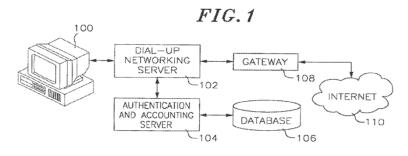
18. In such a conventional ISP environment, a user accesses the Internet by connecting to the ISP, at which point networking software at the user end and the
