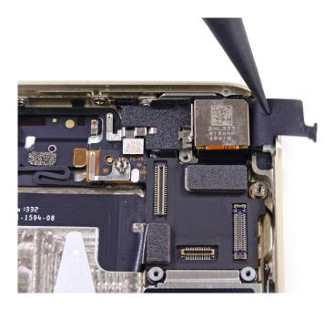
The back of the camera is labeled DNL333 41WGRF 4W61W. According to Chipworks, "the DNL markings are consistent with the markings on the camera modules housing the Sony IMX145 we saw in the iPhone 4s and on the iPhone 5. The marks on the side of the module are different, but our industry insiders tell us this is Sony's again." The bottom of the camera is labeled AW32 65BD 4511 b763.
