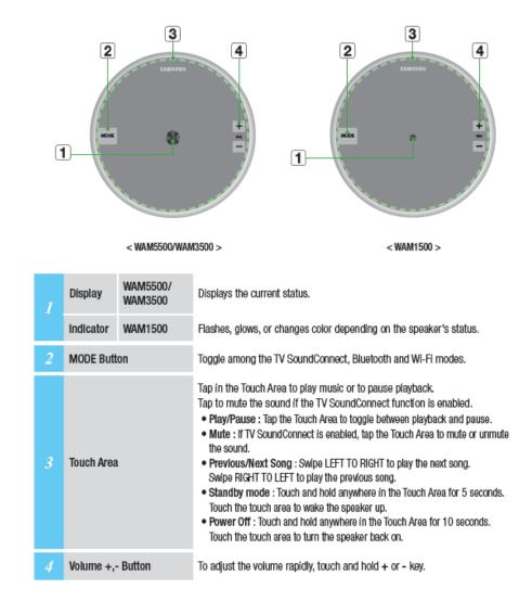
Speaker User Manual at p. 9. For example, if the touch area on the Samsung Radiant360 R1 speaker is swiped from left to right to play the next song, a control signal will be generated and transmitted to the Galaxy S9 via Bluetooth and the Galaxy S9 will broadcast the next song to the Samsung Radiant360 R1 speaker, which will receive and playback the song.
