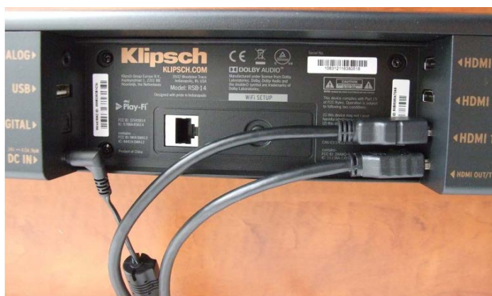
Note that the HDMI 2.0 connectors are compatible with HDCP 2.2. As such, they handle 4K UHD video stream, which they convey without processing (Passthrough) from the source to the display.
