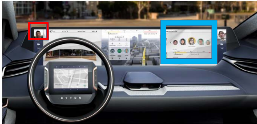
17 A "shared experience display", or SED, replaces the car's interior dashboard, showing 18 content through multiple display screens.
