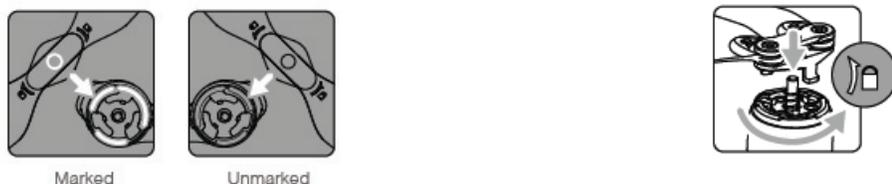
The Spark User Manual also clearly shows the notches of the shaft lock portion and the lugs on the blade lock portion:
