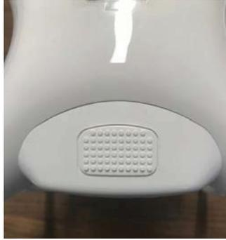
**Figure 28. Clamp Button on DJI Phantom 4 Pro**
