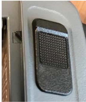
**Figure 33. Restorable Elastic Piece and Clamp Button on DJI Spark**
