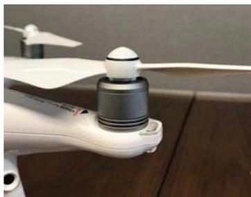
**Figure 22. Propulsion Assembly Comprised of a Propeller and Motor on the DJI Phantom 4 Pro**
