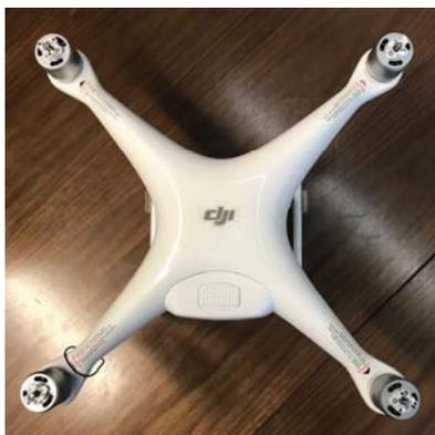
**Figure 19. DJI Phantom 4 Pro (top view) Showing Four Arms Coupled to the Main Body of the UAV**
