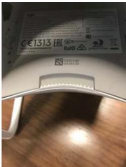
**Figure 34. Clamping Portion on the UAV Body of the DJI Phantom 4 Pro**
