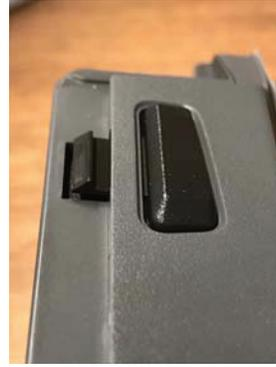
**Figure 32. Restorable Elastic Piece and Clamp Button on DJI Mavic Pro**
