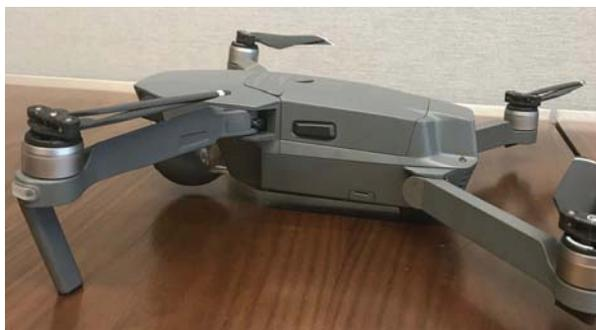
**Figure 14. DJI Mavic Pro (side view) with Battery Inserted**
