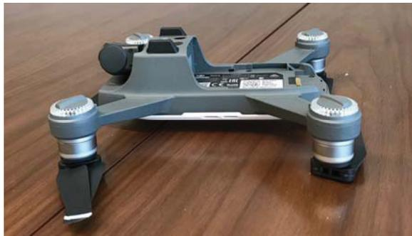
**Figure 18. DJI Spark (side view; upside-down) with Battery Removed**
