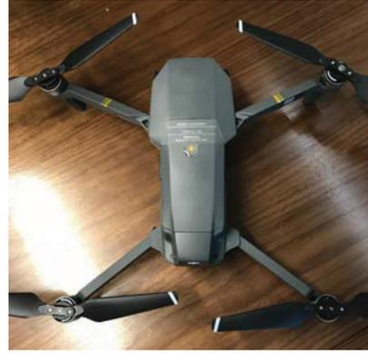
**Figure 20. DJI Mavic Pro (top view) Showing Four Arms Coupled to the Main Body of the UAV**
