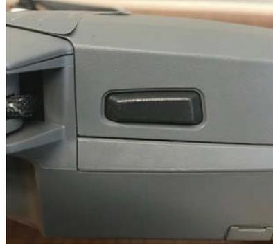
**Figure 29. Clamp Button on DJI Mavic Pro**
