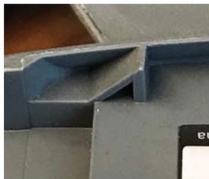
**Figure 36. Clamping Portion on the UAV Body of the DJI Spark**
