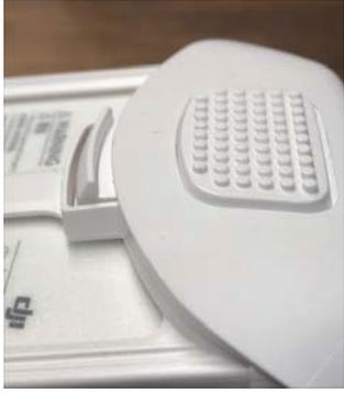
**Figure 31. Restorable Elastic Piece and Clamp Button on DJI Phantom 4 Pro**
