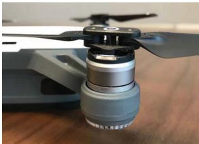
**Figure 24. Propulsion Assembly Comprised of a Propeller and Motor on the DJI Spark**
