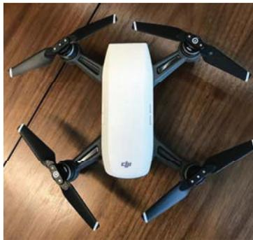
**Figure 21. DJI Spark (top view) Showing Four Arms Coupled to the Main Body of the UAV**
