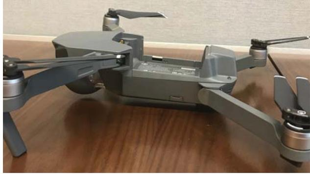
**Figure 16. DJI Mavic Pro (side view) with Battery Removed**
