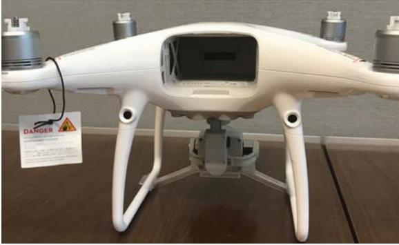
**Figure 15. DJI Phantom 4 Pro (rear view) with Battery Removed**
