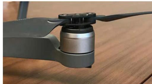
**Figure 23. Propulsion Assembly Comprised of a Propeller and Motor on the DJI Mavic Pro**
