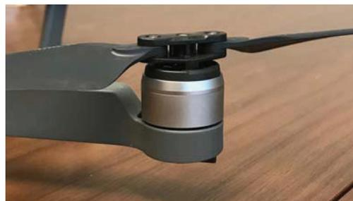
**Figure 23. Propulsion Assembly Comprised of a Propeller and Motor on the DJI Mavic Pro**
