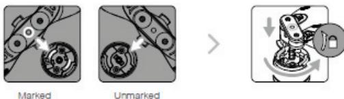
The Phantom 4 User Manual also shows the notches that would attach to the lugs on the blade lock portion:
