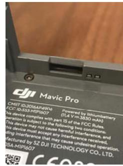
**Figure 35. Clamping Portion on the UAV Body of the DJI Mavic Pro**
