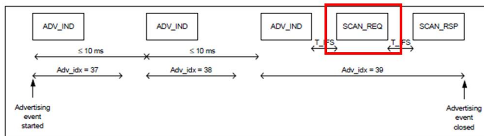
Figure 4.9: Connectable and scannable undirected advertising event with SCAN_REQ and SCAN_RSP PDUs at the end of an advertising event
