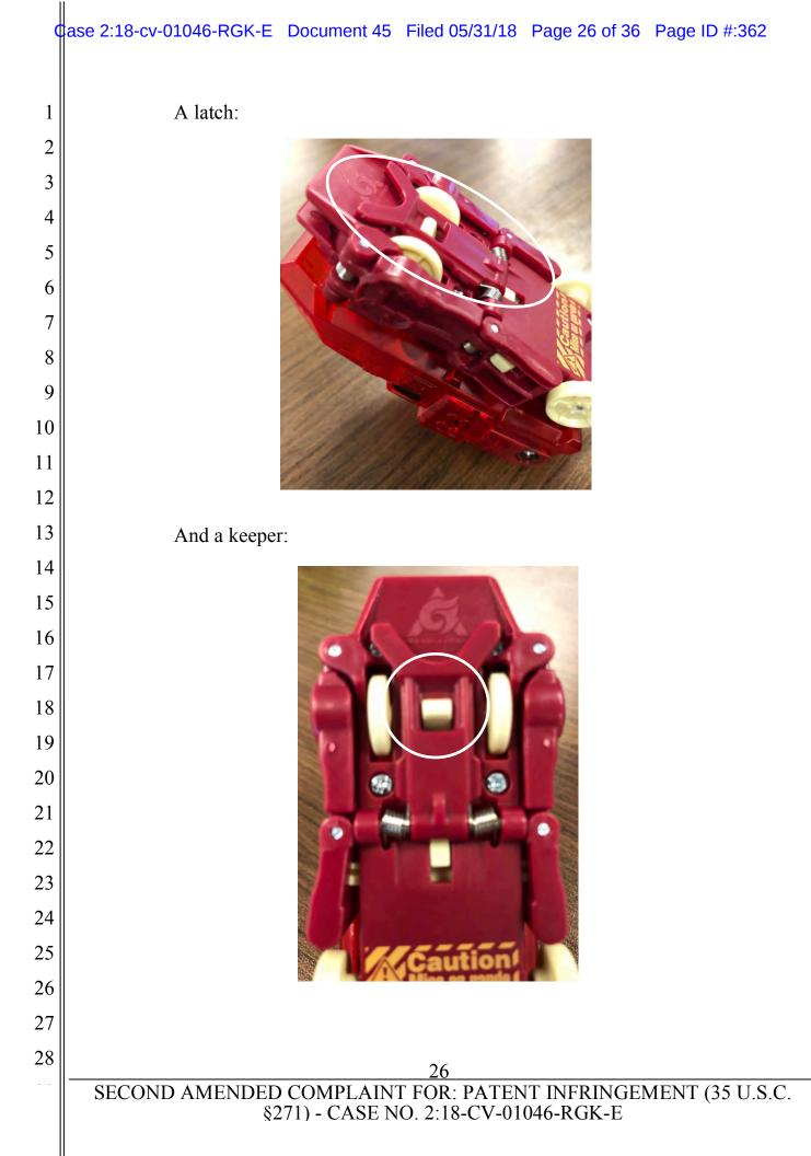
53. For each Screechers Wild! toy, the elastic element urges the locking assembly towards a locking position in which the latch and the keeper are engaged with one another and at least indirectly retain the at least one auxiliary component in the first position:
