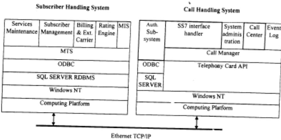
**Figure 1: NetManager Software Architecture**
