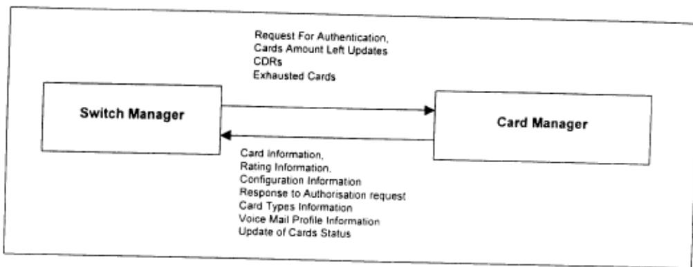
**Figure 3: Dataflow between Switch Manager and Card Manager**
