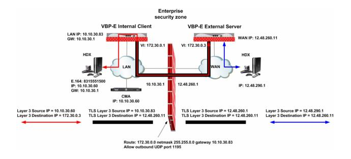
In the above diagram, a "VBP-E Internal Client" is located inside an enterprise firewall; a "VBP-E External Server" is located outside an enterprise firewall; and all audio and video communication between the local and remote "HDX" communication devices is sent through a secure tunnel formed between the "VBP-E Internal Client" and the "VBP-E External Server."
