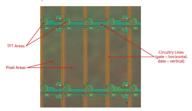
16. A TFT acts as a switch that operates its respective individual pixels using the circuity lines. In that way, the pixels can be turned on and off to create an image on an LCD by allowing or preventing light to pass through. The individual pixels are more apparent when a color filter layer overlays the circuits as shown in the image below for the M270HGE-L30.
