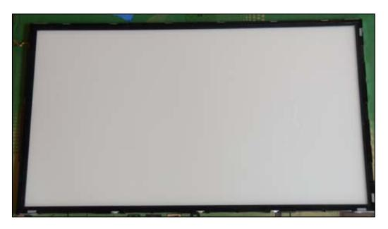
16. A TFT-LCD panel's backlight module contains many components. The image below shows, for example, part of the backlight module's tray, and its transparent light guide panel
