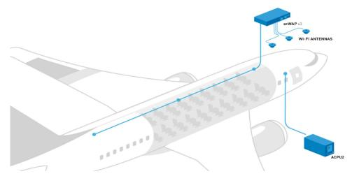
that aircraft are equipped with "ACPU-2," described as a "[n]ext-generation onboard server unit that uploads and downloads data to the aircraft both inflight and on the ground. *See* "In-Cabin Network Hardware for inflight connectivity and entertainment," https://www.gogoair.com/commercial/in-cabin-network.
