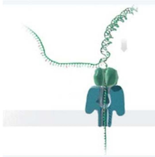
Exhibit 7. As the DNA passes through the hole, it disrupts the electrical current that is passing through the hole, thus producing a signal. To evaluate the sequence, one can attempt to correlate this signal with the DNA bases that are passing through the hole.
