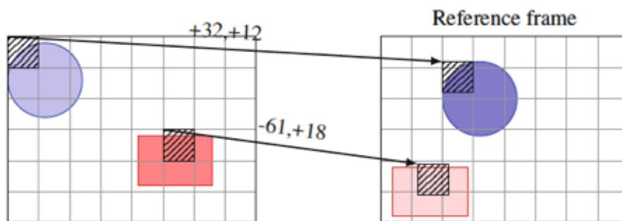
Fig. 2.4: Motion estimation. For each MB the best matching block in the reference frame is found. The encoder codes the differences (errors) between the MBs and their best matching blocks. Arrows indicate motion vectors and are labeled by the vector coordinates. In this example the shapes are identical but their colors are slightly larger/darker.
