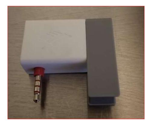
22. The connector in the MCR System bridges a microphone pin of the audio input port such that the mobile device detects a presence of the connector in the audio input port. *See*, e.g., **3.5 mm jack circuit**. An example is illustrated below:
