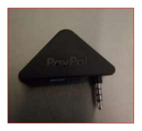
22. The connector in the MCR System bridges a microphone pin of the audio input port such that the mobile device detects a presence of the connector in the audio input port. *See*, e.g., **3.5 mm jack circuit**. An example is illustrated below:
