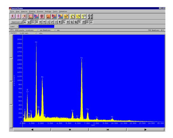
The spectrum below from the "Spectrum 2" area indicates that the powder particles dispersed in the resin are predominantly iron (element "Fe"), indicating that a magnetic powder is dispersed in the polymer resin.
