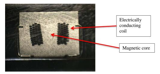
The primary elements present in the inductor core, as indicated by the spectrum below, are iron, chromium, and silicon. The inductor core is predominantly iron, a magnetic substance. Accordingly, the core is magnetic.
