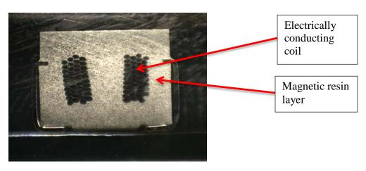
15. The magnetic resin layer contained in the Accused Products contains a magnetic powder dispersed in a polymer resin. The photograph below depicts a cross section of the composition of the resin material, and shows that the resin material comprises a powder dispersed in the resin. The spectrums below detail the components of the magnetic resin layer. Spectrum 3 indicates the presence of the polymer resin. Spectrum 2 indicates the presence of a ferromagnetic metal powder, iron (Fe).
