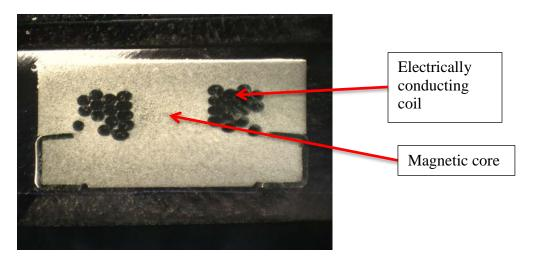
The primary elements present in the inductor core, as indicated by the spectrum below, are iron, chromium, and silicon. The inductor core is predominantly iron, a magnetic substance. Accordingly, the core is magnetic.
