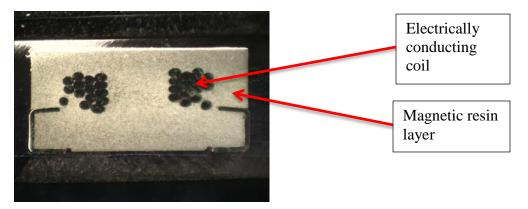
15. The magnetic resin layer contained in the Accused Products contains a magnetic powder dispersed in a polymer resin. The photograph below depicts a cross section of the composition of the resin material, and shows that the resin material comprises a powder dispersed in the resin. The spectrums below detail the components of the magnetic resin layer. Spectrum 3 indicates the presence of the polymer resin. Spectrum 2 indicates the presence of a ferromagnetic metal powder, iron (Fe).
