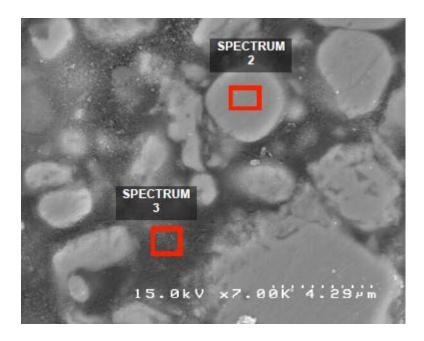
The spectrum below from the "Spectrum 3" area indicates that the resin material is substantially aluminum (element "Al"), indicating that the resin material is a polymer aluminum resin.
