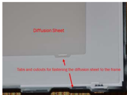
Diffusion Sheet detached from Frame
