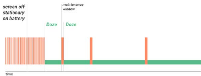
Figure 1. Doze provides a recurring maintenance window for apps to use the network and handle pending activities.
