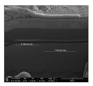
184. Focusing in on a portion of the above side surface, a metal layer is shown covering a portion of the distributed Bragg reflector to reflect light transmitted through the distributed Bragg reflector.
