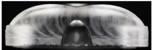
91. Two images are provided below. The left and right images show a side view of a light source from the RCA LED TV LED55C55R120Q television created using a microscope and scanning electron microscope. The light source has a width of approximately 3 millimeters.
