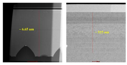
148. The transmission electron microscope image below further enlarges the multiquantum well active region, which comprises a plurality of quantum dot layers separated by a plurality of barrier layers. The plurality of quantum dot layers appear as relatively thin and bright layers separated by relatively thick and dark barrier layers.
