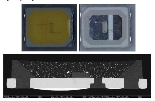
113. The images show the LED mounted on the body of the package and connected to leads. The light emitting diode chip is shown covered by a member comprised of resin. The resin member contains phosphor particles, which can be seen as relatively bright spots within the darker resin.
