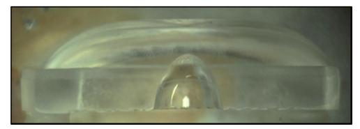
76. As the above image shows, the substantially vertical portions of the side surfaces, which comprise part of the light exit plane, are textured, resulting in protrusions extending above the surface of the lens. The side surface of the lens also includes a curved surface.
