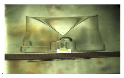
68. Below is an image of a cross-section through a lens removed from a RCA LED TV LED24G45RQ television. The lens comprises a solid of revolution of the cross-section around the central axis of the lens.
