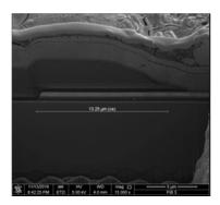
159. The image below shows an electron microscope image of the side surface of a hole milled into the light emitting diode chip removed from the 55PFL5402/F7 television. The top of the image shows multiple layers of a protective insulation layer covering a sidewall of the first conductive type semiconductor layer and the second conductive type semiconductor layer.
