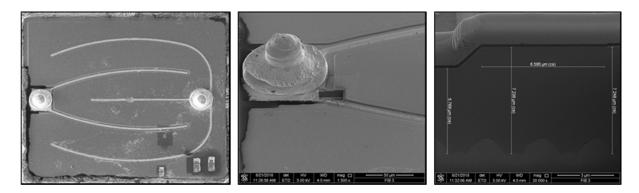
136. The p-type semiconductor layer of the LED comprises a number of layers. From top to bottom, the layers include a p-type contact layer, a hole transport layer, and a hole injection
