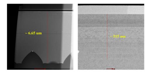
143. Based on the level of Indium doping in the active region, the superlattice layer, and the spacer layer, the spacer layer will have a bandgap smaller than the barrier layers of the multiquantum well, but higher than the bandgap of the quantum well layers.
