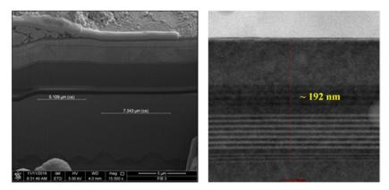
167. The image below left again shows the side surface of the milled hole. The image below right focusses in on the center of the far right side of the left image. The bottom layer in the image below right is a portion of the second semiconductor layer. Above the second semiconductor layer is a reflection pattern.
