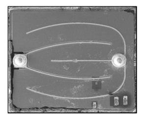
128. The n-pad of the LED is shown as a circular structure toward the center of the left side of the image. The n-pad is formed over an n-type semiconductor layer. The P-pad of the LED is shown as a circular structure toward the center of the right side of the image. The P-pad is formed over a p-type semiconductor layer.
