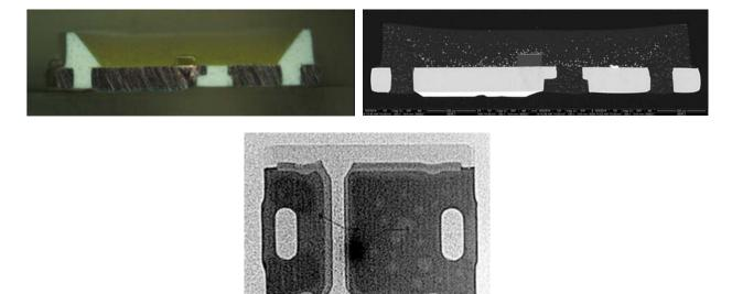
51. The images above depict a pair of spaced-apart lead frames, each having an upper and lower surface. Each of the lead frames also includes sidewalls that connect the upper and lower surfaces. All three images show a light-emitting diode chip on the top surface of the left lead frame.
