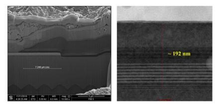
156. The image below shows the locations of a plurality of contact holes that extend through the first conductive type semiconductor layer and active layer of a light emitting diode chip removed from the 55PFL5402/F7 television. The plurality of holes expose the second conductive type semiconductor layer.
