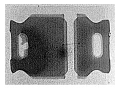
45. The images above depict a pair of spaced-apart lead frames, each having an upper and lower surface. Each of the lead frames also includes sidewalls that connect the upper and lower surfaces. All three images show a light-emitting diode chip on the top surface of the left lead frame.
