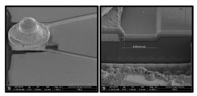
61. As the above top-surface view of the light emitting diode shows, two n-extensions extend from the n-electrode pad toward the right edge. The far right ends of the n-extensions are further apart than the far left ends that connect to the n-electrode pad. The top n-extension is convexly bent towards the top edge and the bottom n-extension is convexly bent toward the bottom edge.
