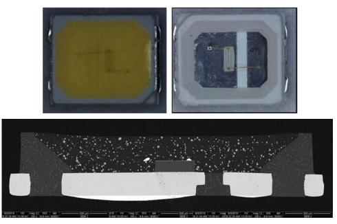
120. The cross-section image above show the LED covered by a member comprised of resin. The resin member contains phosphor particles, which can be seen as relatively bright spots within the darker resin.
