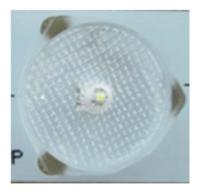
97. Two images are provided below. The top image is a side-view of a lens from the RCA LED TV LED55C55R120Q television. The bottom image was taken after a lens was cross-sectioned. As the images show, the lens has a concavity at its center. The surface of the concavity forms a light incident surface. The images below also show the upper surface of the lens through which light is emitted.
