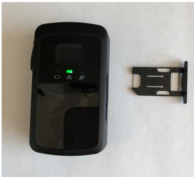
*Figure 8. The Optimus Mini GPS Tracker receives one location point per minute and store the location point in its memory if it cannot communicate with the server, based on a lack of cellular coverage, which was found by removing the SIM card.*
