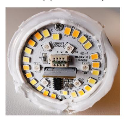
36. The Accused Infringing Devices contain a substrate, a cluster of LED chips, which are arranged two-dimensionally on the substrate and a plurality of phosphor resin portions that cover the respective LED chips.
