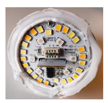
The Accused Infringing Devices contain a substrate, a cluster of LEDs, 24. which are arranged two-dimensionally on the substrate and an interconnection circuit which is electrically connected to the LEDs.
