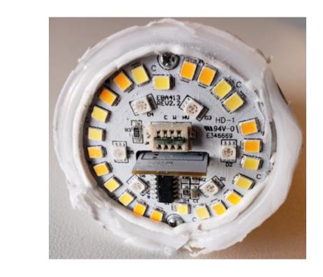
13. The Accused Infringing Devices have a blue LED for producing an emission wavelength falling within a blue wavelength range. Exemplary blue LEDs, which are covered in a yellow phosphor, can been seen in the picture of an Accused Infringing Device below.
