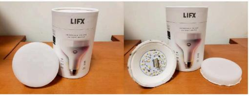
14. The Accused Infringing Devices have a blue LED for producing an emission wavelength falling within a blue wavelength range. Exemplary blue LEDs, which are covered in a yellow phosphor, are shown circled in red in the figures below.
