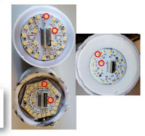
material used in LEDs is illuminated by blue light, it emits yellow light having a fairly broad spectral power distribution. By incorporating the phosphor in the body of a blue LED with a peak wavelength around 450 to 470 nanometers, some of the blue light will be converted to yellow light by the phosphor. The remaining blue light, when mixed with the yellow light, results in white light. New phosphors are being developed to improve color rendering as shown in Figure 5.
