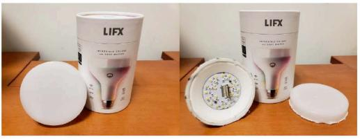
24. The Accused Infringing Devices contain a substrate, a cluster of LEDs, which are arranged two-dimensionally on the substrate and an interconnection circuit which is electrically connected to the LEDs.
