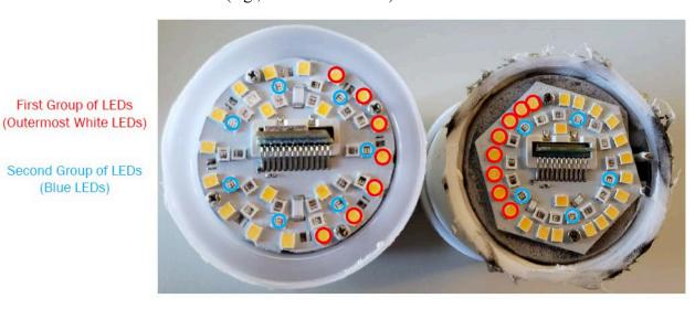
26. The Accused Infringing Devices contain an interconnection circuit wherein the interconnection circuit has an interconnection structure for separately supplying drive currents to at least one of the LEDs in the first group and to at least one of the LEDs in the second group separately from each other. One or more of the LEDs in the outer periphery can be operated independently of one or more LEDs located toward the center.
