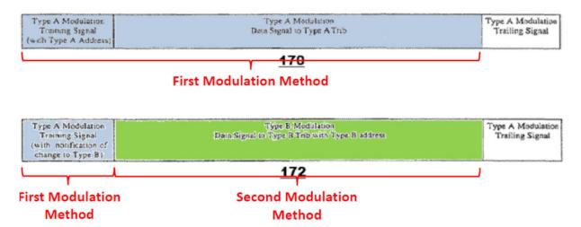
'228 Patent at Fig. 8, 4:45-48, 4:66-5:1. Information in the training signal indicates whether there will be an impending change from the first type of modulation method to the second type of modulation method. *Id.* (training signal includes "notification of change to Type B" modulation method).
