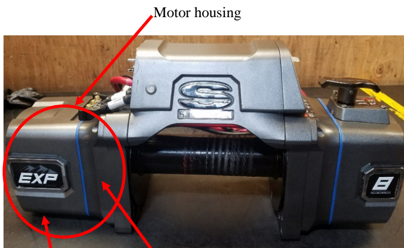
5 First drum support directly coupled to and closing said motor case
