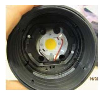
28. On information and belief, Yori Track Large 30W products include a heat dissipation element thermally coupled to the thermally conductive substrate; for example, a heat dissipation element, formed by a metal backing (shown above) and fins (shown below), is thermally coupled to the PCB.
