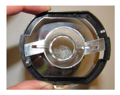
The PCB is enclosed between the metal backing and the recessed optic when the recessed optic and twist-lock fixing ring are fastened to the metal backing. The recessed optic includes a transparent lens enabling transmission of light emitted by the LEDs therethrough.
