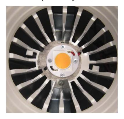
80. On information and belief, Rollios 13W products include a first reflector having said first aperture disposed in an upper portion of said first reflector and an opposed larger second aperture in a lower portion of said first reflector; for example, the array of LEDs are positioned adjacent a first aperture of a multi-piece reflector assembly including a first reflector,
