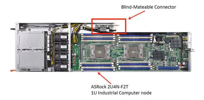
42. Furthermore, the ASRock 2U4N-F2T units are remotely monitored industrial computers because ASRock provides hardware and software for remotely monitoring its devices. For example, the 2U4N-F2T servers include Management features, such as the ASPEED AST2400 BMC Controller.<sup>4</sup>
