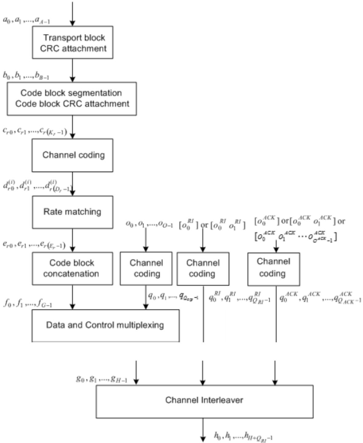
Figure 5.2.2-1: Transport channel processing for UL-SCH
