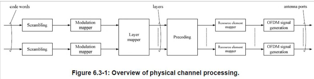
Figure 6.3-1: Overview of physical channel processing.
