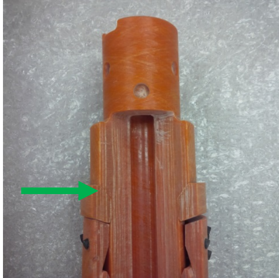
Proximate end with angled transition surface
