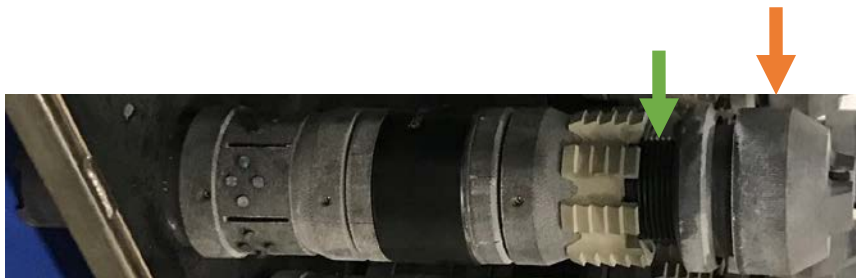
Lower sleeve (orange arrow) around a set of threads (green arrow)
