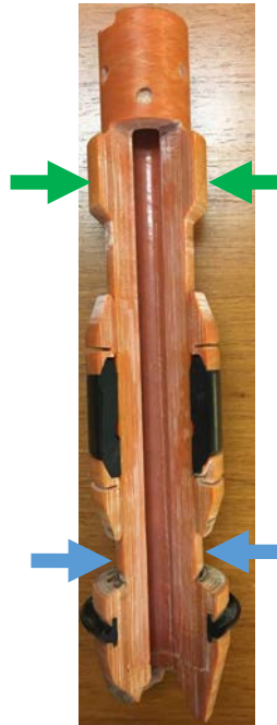
Proximate end with larger diameter (green arrows)
