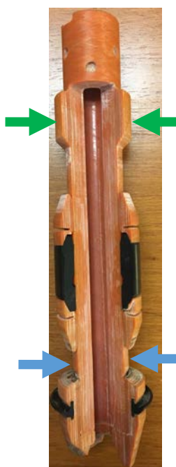
Proximate end with larger diameter (green) than distal end (blue)
