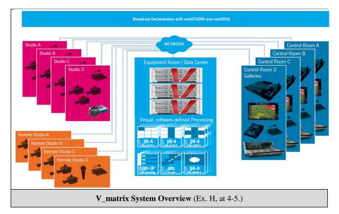
55. The accused product comprises a master controller that generates input processor control signals and output processor control signals. For example, vsmSTUDIO and/or vsmSOUL provides a "unified orchestration, control and monitoring system" that generates input processor control signals and output processor control signals. The accused product accomplishes IP routing using vsmSOUL:
