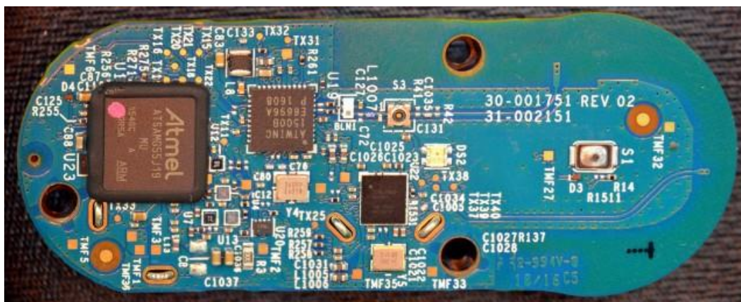
Teardown picture showing Amtel ATWINC1500B Wi-Fi module. https://mpetroff.net/2016/07/new-amazon-dash-button-teardown-jk29lp/#f1-2185
