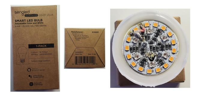
23. The Accused Infringing Devices contain a substrate, a cluster of LEDs, which are arranged two-dimensionally on the substrate and an interconnection circuit which is electrically connected to the LEDs.
