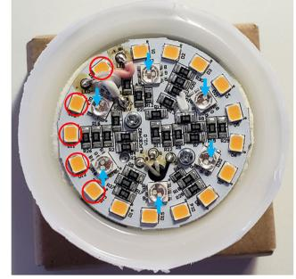
First Group of LEDs (White LEDs) Second Group of LEDs (Blue LEDs)
