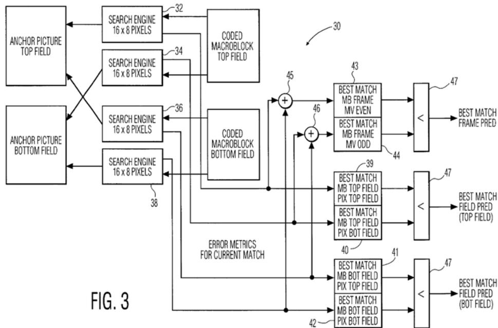
28. Claim 1 of the '005 patent improves the functionality of motion coding in video compression by performing the concurrent determination of the optimal prediction mode while performing motion estimation along with generating the motion vector. The claimed invention of claim 1 of the '005 patent also was not well-understood, routine or conventional at the time of the invention. Rather, as set forth below, the claimed invention was a departure from the
