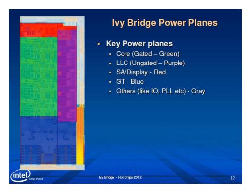
57. The on-chip power gates can only reduce the core (first) voltage from the supplied VCC power rail. When the core voltage (the first voltage) is above the operating voltage of the memory, the power gate will be fully opened, and the first voltage (core voltage) and the second voltage (VCC) will be the same. Thus, when the first voltage is above the minimum operating voltage of the memory, the first voltage will be provided to the memory array.
