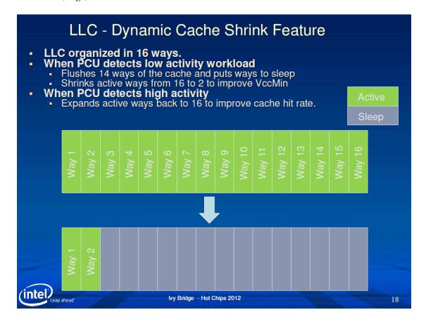
["increasing the power supply voltage to a third value; identifying a second set of ways of the first set of ways that is functional with the power supply being applied at the third value; and accessing the cache including the second set of ways."]
