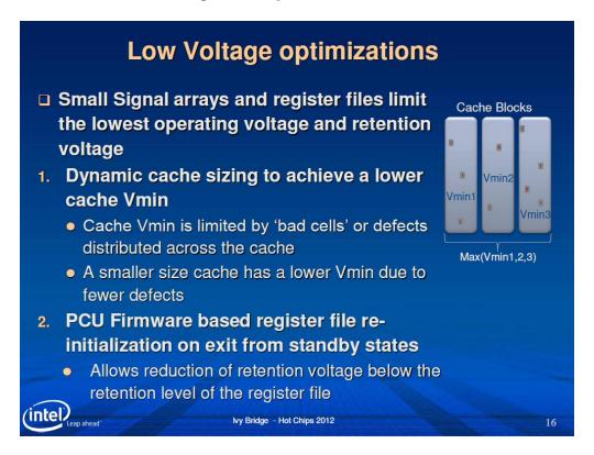
22. The PCU flushes and puts to sleep a subset of the ways, shown here as ways 3-16, that would be non-functional at the lower voltage. *See*, *e.g.*, PM at 16:
